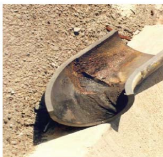
Figure 12—Erosion-Corrosion of Carbon Steel Piping Elbow
